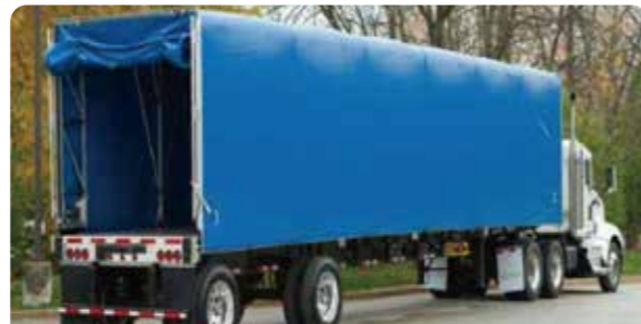
Slipping Vehicle Tarpaulin System Assembly
